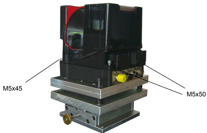
Figure 17 Measurement device attached to the deluxe mounting system
